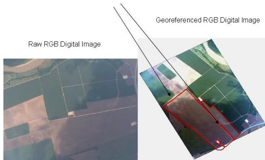
Figure 7. RGB digital image and georeferenced image with overlay of GIS polygon of the big pivot west field.
